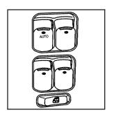
The power window switches are located on the armrest on the driver's door. In addition, each passenger door has a switch for its own window.
